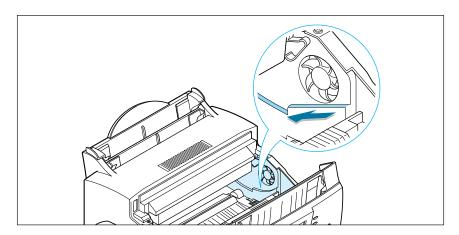
5. Grasp the handle at the front of the cartridge and slide it down between the cartridge slots, and push it firmly.
